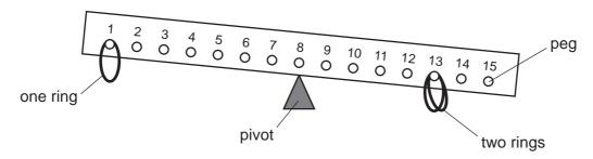
The wooden rod is uniform and all the rings are of equal mass. Two rings are hung on peg 13 and one on peg 1.
