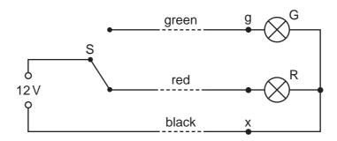
The signal is some way from S to which it is connected by a cable with green, red and black wires. At the signal, the green and red wires are connected to the corresponding lamp and the black wire is connected to a terminal x to provide a common return. The arrangement is shown correctly connected and with the switch set to illuminate the red lamp.
