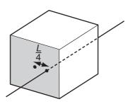
When viewing the shaded face, what is the torque of the couple that will now be needed to stop the cube from toppling?
