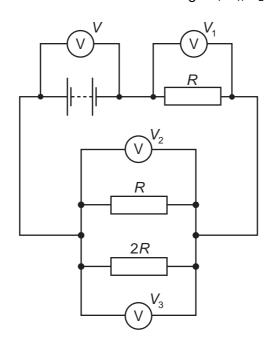
Which equation relating the voltmeter readings must be true?
