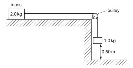
What is the speed of the 2.0 kg mass as the 1.0 kg mass hits the floor, having fallen a distance of  $0.50\,m$ ?
