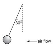
The ball is suspended by a light string and weighs 0.15 N.
