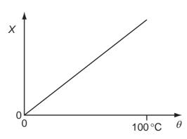
$\theta$  is determined from the corresponding values of X by using this graph. X is measured with a percentage uncertainty of  $\pm 1$  % of its value at all temperatures.
