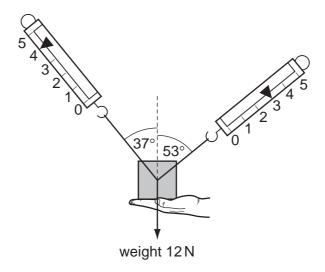
When the person's hand is removed, what is the initial vertical acceleration of the mass?
