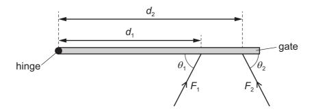
One person is distance  $d_1$  from the gate's hinge and pushes with horizontal force  $F_1$  at angle  $\theta_1$  to the gate.
