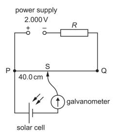
The potentiometer wire PQ is 100.0 cm long and has a resistance of  $5.00 \Omega$ . The power supply has an e.m.f. of 2.000 V and the solar cell has an e.m.f. of 5.00 mV.
