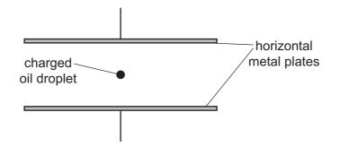
As some of the oil evaporates, the droplet loses mass and starts to accelerate. Its charge remains constant.
