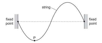
The frequency of the wave is 250 Hz. Point P on the string has a vertical displacement of -1.0 mm.
