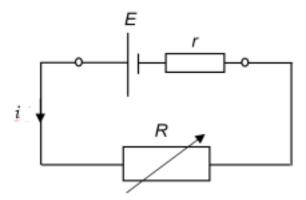
The resistance *R* of the variable resistor is decreased so the current *i* in the circuit increases. This eliminates **B** as a possible answer.
