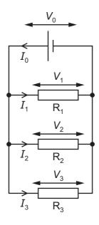
Which equation can be obtained by applying Kirchhoff's second law to the circuit?
