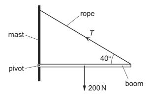
The rope is at an angle of  $40^{\circ}$  to the horizontal and exerts a tension force T on the boom. The weight of the boom is 200 N. The mass of the boom is uniformly distributed along its length. The boom is in equilibrium.
