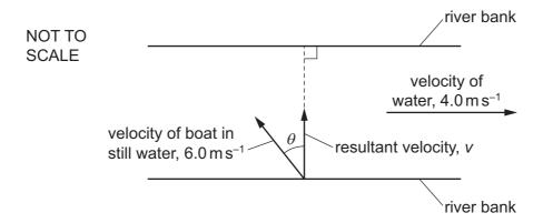
In still water, the speed of the boat is  $6.0\,\mathrm{m\,s^{-1}}$ . The boat is directed at an angle  $\theta$  to a line perpendicular to the river banks. The resultant velocity v of the boat is in a direction perpendicular to the river banks.
