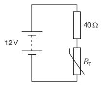
Initially, the temperature of the thermistor is 15 °C and the current in the circuit is 0.10 A.
