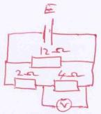
The voltmeter has a very high resistance and reads a potential difference  $V_{\rm out}$ .
