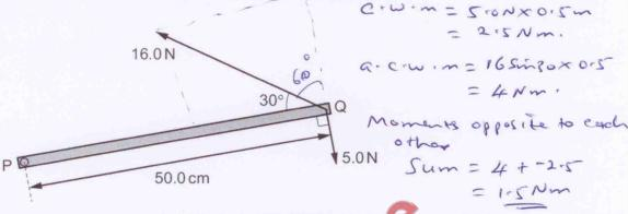
Two forces of 16.0 N and 5.0 N are in the horizontal plane and act on end Q as shown in the diagram.
