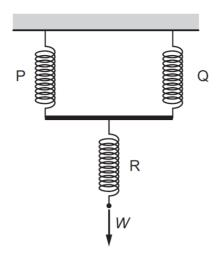
Springs P and Q are identical and each has spring constant k. Spring R has spring constant 3k.
