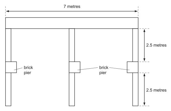
A double-brick-wide wall needs 120 bricks per vertical square metre. A single-brick-wide wall needs 60 bricks per vertical square metre. Brick piers need 14 bricks per vertical metre.
