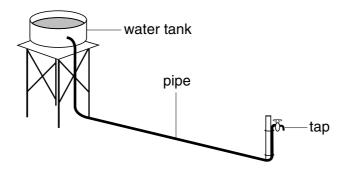
(Rate of flow through pipe = speed of flow  $\times$  cross-sectional area of pipe.)
