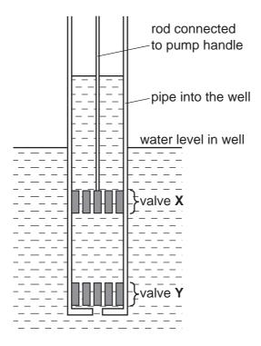
Which valves move or remain stationary as the water is pumped?
