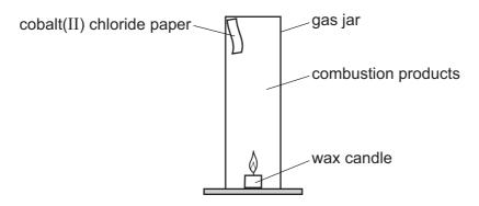
After a short time, the oxygen in the jar is used up and the candle flame goes out.
