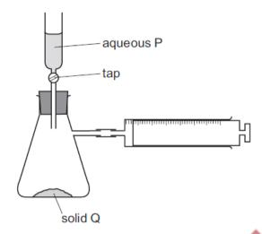
A small volume of aqueous P is poured on to solid Q and the tap of the funnel closed.
