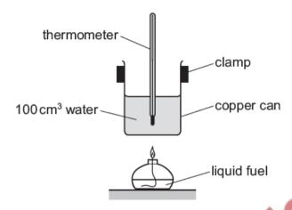
All conditions are kept the same apart from the type of fuel and mass of fuel burned.
