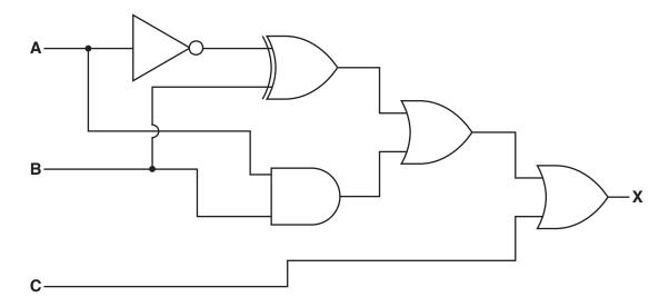
(a) Complete the truth table for the given logic circuit.
