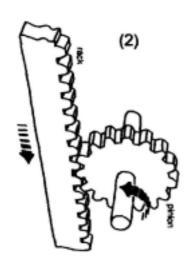
Rack and pinion (1) converts rotary into linear motion (1).
