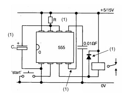
(b) Interface (1) between two circuits of differing current rating (1). Control of large current by small current device (1).
