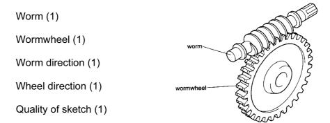
(ii) The VR of the system is large (1) as the worm (driven gear) has effectively one tooth (1).
