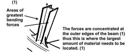
(ii) Joists in a building structure. [1]
