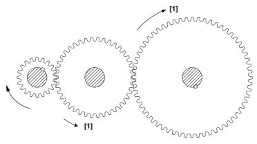
(ii) Gear ratio is 3:1, gear C rotates at 20 rpm.
