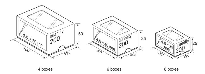
Design a unit that would hold the size and quantity of screw boxes shown so that they can be easily accessed. The unit could be positioned anywhere in the school workshop.
