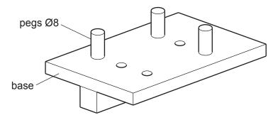
Complete Table 2.1 by giving the missing stages required to braze the pegs into the base.
