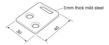
(f) Fig. 11.5 shows details of a shelf that is to be fitted to the legs of the table at the height shown.
