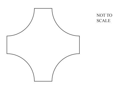
This shape is made from four straight edges and four arcs. Each straight edge has length 3 cm. Each arc is a quarter of the circumference of a circle of radius 5 cm.
