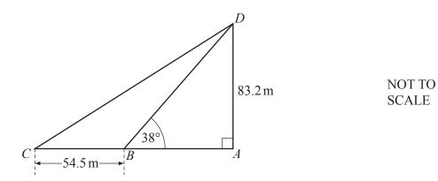
ACD is a right-angled triangle. B is on AC and BC = 54.5 m.  $AD = 83.2 \,\text{m}$  and angle  $ABD = 38^{\circ}$ .
