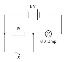
What happens to the brightness of the lamp when switch S is closed?
