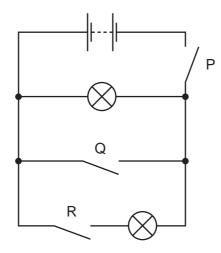
Which switches must be closed so that both lamps will light?
