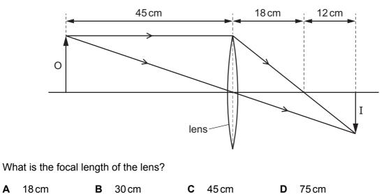
**30** The diagram shows light from an object O passing through a converging lens to form an image I.
