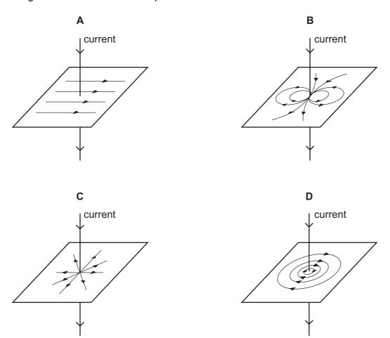
36 A student carries out an experiment to see the effect of a magnetic field on a will current.
