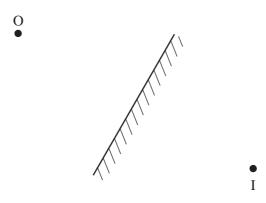
If the object moves towards the mirror in the direction shown by the arrow, in which direction does the image move?
