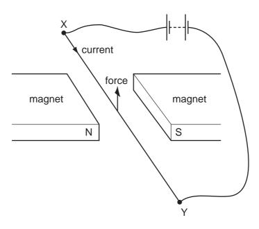
If the north and south poles of the magnet exchange positions, in which direction will the force on the wire act?
