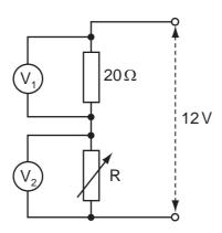
When R has a value of  $20 \Omega$ , the voltmeter readings are equal.
