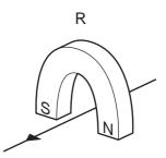
current direction reversed and magnet turned around
