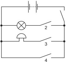
Which switches must be closed for the bell to ring without lighting the lamp?
