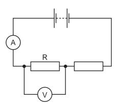
The reading on the ammeter is 2.0 A and the reading on the voltmeter is 8.0 V.
