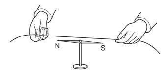
An electric current is switched on in the wire and the compass needle is deflected.
