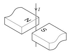
What is the direction of the force on the wire exerted by the magnetic field?
