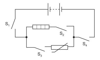
Which three switches must be closed for the heater to work?
