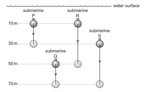
Which row is correct for the difference in pressure from the initial to the final depth of each submarine?
