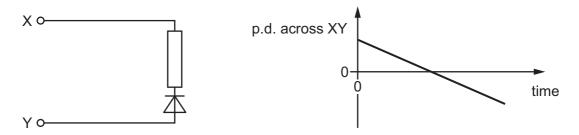
Which graph shows how the current in the circuit (from X to Y) varies during the same time interval?
