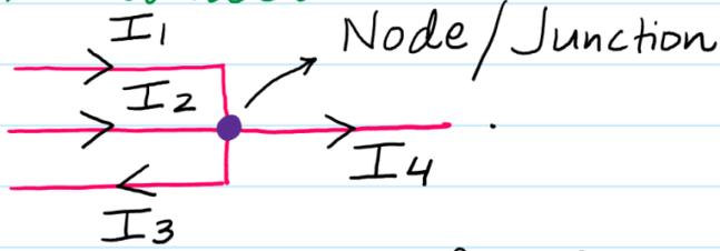
form an equation for Current based on KCL
