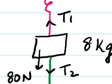
$$\begin{aligned} T_2 &= 20 \text{ N} \\ T_1 &= 100 \text{ N} \end{aligned}$$
