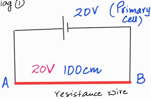
\* Diag 1 shows a resistance wire AB which is connected to a 20V battery (Primary cell). Length of wire AB = 100cm. Connecting wires have Zero Resistance
