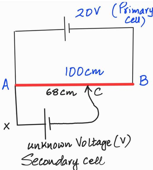
Q: Given that a null deflection / Zero Current / Balance pt is achieved for length AC = 68cm. Use this info. to calculate the unknown Voltage (V) of the Secondary cell.
