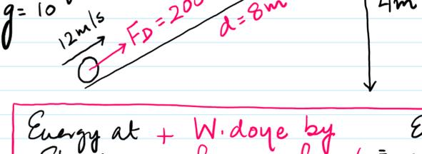
③ Energy at Start + W. done by forward force/ driving force/ Engine = Energy at End.
