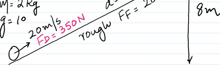
④ Energy at Start + W.d by Engine - W.d against friction = Energy at End
