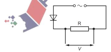
Which graph shows how the voltage *V* across the resistor R varies with time?
