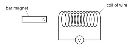
The N-pole of the magnet is moved quickly towards the coil. The voltmeter shows a reading of +10 mV.
