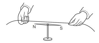
An electric current is switched on in the wire and the compass needle is deflected.
