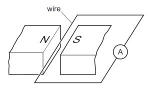
The wire is moved downwards, towards the bottom of the page. A current is induced in the wire.
