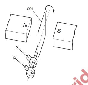
Diagram 2 shows the output voltage produced by the generator as the coil turns.
