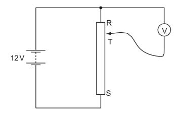
What happens to the reading on the voltmeter as the sliding terminal T is moved from R to S?
