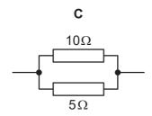
The total resistance is less than  $5\Omega$ .
