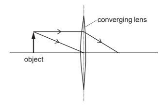
An image of the object is formed on a screen to the right of the lens.
