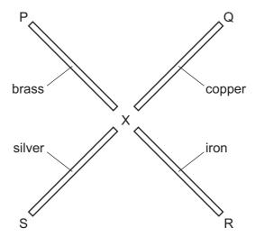
Wax is used to attach small metal balls at the rod ends P, Q, R and S.
